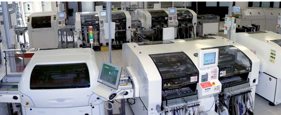
INTERNAL VIEW OF CEIA SMT (SURFACE MOUNTING TECHNOLOGY) DEPARTMENT
